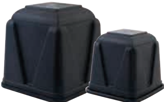
VANTAGE® 71010463 BLACK VAULT LARGE Outside Dimensions: 18" H x 18" W x 18" D Inside Dimensions: 15.375" H x 15.375" W x 15.375" D load tested up to 5,000 lbs per square foot VANTAGE® 71010461 BLACK VAULT MEDIUM Outside Dimensions: 13.75" H x 13.5" W x 13.5" D Inside Dimensions: 12.75" H x 12" W x 12" D load tested up to 5,000 lbs per square foot
