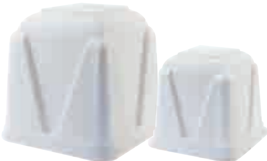
VANTAGE® 71010464 WHITE VAULT LARGE Outside Dimensions: 18" H x 18" W x 18" D Inside Dimensions: 15.375" H x 15.375" W x 15.375" D load tested up to 5,000 lbs per square foot VANTAGE® 71010462 WHITE VAULT MEDIUM Outside Dimensions: 13.75" H x 13.5" W x 13.5" D Inside Dimensions: 12.75" H x 12" W x 12" D load tested up to 5,000 lbs per square foot
